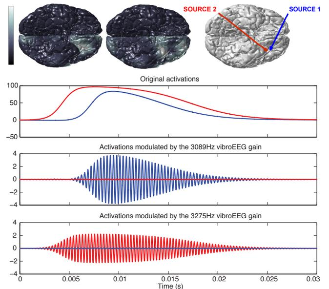
**Fig. 1.** First row: vibrational mode of the CC for frequencies 3089Hz (left) and 3275Hz (middle), and the locations of the simulated sources on the CC (right). Second row: simulated activations of the sources (in nAm). Third and fourth rows: vibroEEG-modulated source voltages (in microvolts) recorded at the 'Fp1' electrode for both frequencies.
