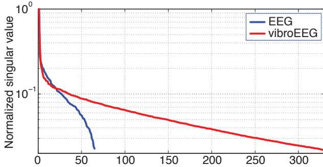
**Fig. 2.** Singular values corresponding to the vibroEEG gain matrix (red) based on 400 modes and sampled at 65 points of the 10–20 system vs the singular values of the corresponding EEG gain matrix (blue).
