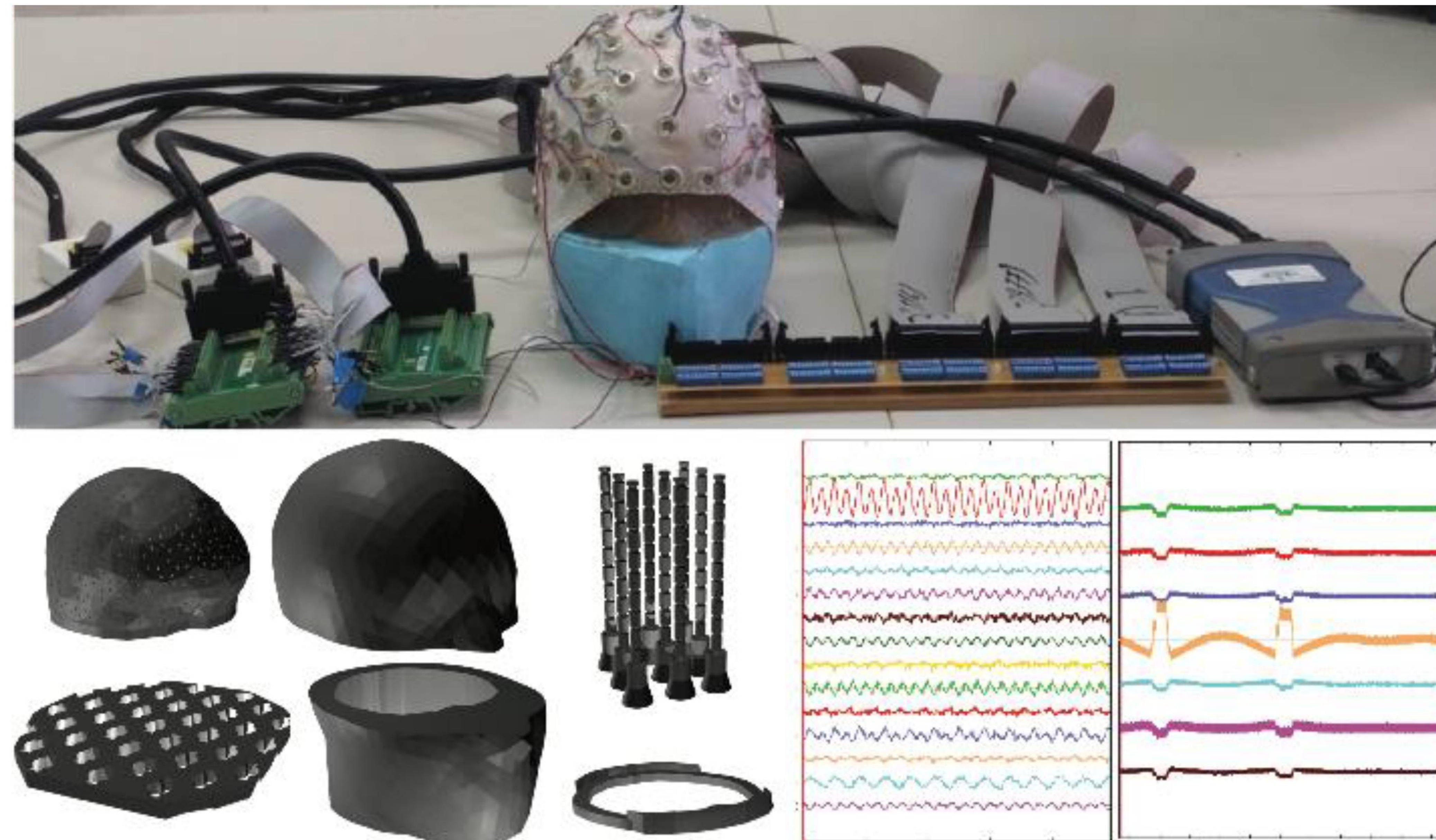
Figure 1: Phantom with connected EEG cap and signal sources and the breakdown of the constituent 3D printed parts. Recorded signals show emulated interference and motion artifacts.
