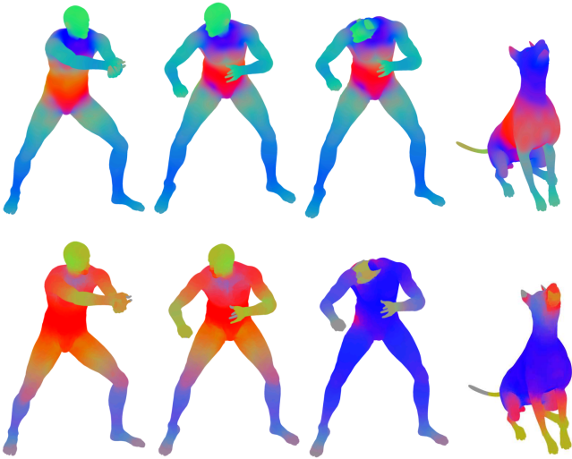
Figure 3: RGB representation of the first three components of the HKS descriptor (first row) and VHKS descriptor on the shape boundary (second row). Second and third columns show, respectively, a volume-preserving and a volume changing boundary isometries.
