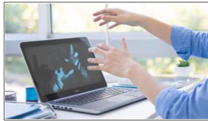
Intel RealSense sensor integrated into a laptop allowing gesture-based interaction. Image credit: Intel.
